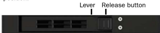
6. Pull the lever carefully to remove the disk from the drive.
