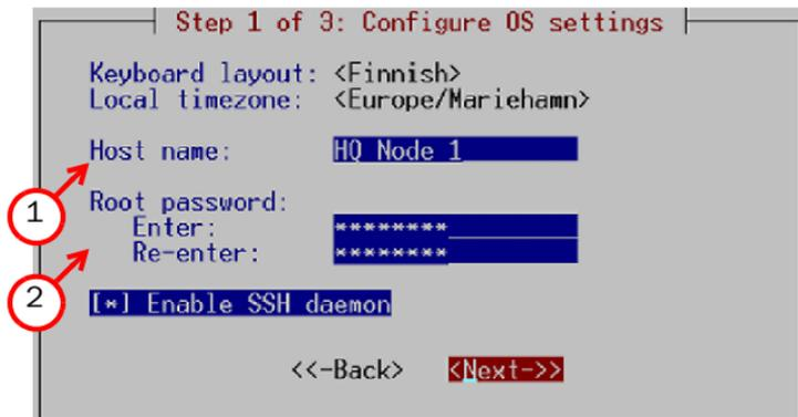
2. Type in the password for the user `root`. This is the only account for engine command line access.
