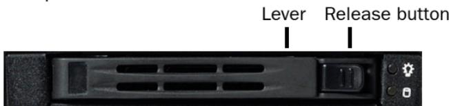
6. Pull the lever carefully to remove the disk from the drive.
