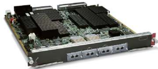
Figure 4. Cisco Catalyst 6500 4-Port 10 Gigabit Ethernet Fiber Module
