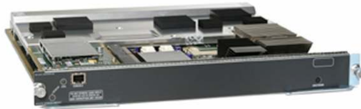
Figure 1. The Cisco WebVPN Services Module
