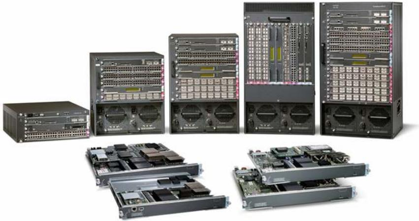
The Catalyst 6500 Series offers a wide range of integrated service modules on a single networking platform. These service modules add Layer 4–7 functionality to the existing Layer 2–3 capabilities of the switch, transforming the Catalyst 6500 Series into a fully functional Layer 2–7 device. The integrated service modules use the high-speed switching backplane and intelligent networking capabilities to:
