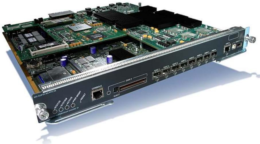
The Supervisor Engine 32-10GE is the second Supervisor Engine 32 option now shipping. It provides two front 10-Gigabit Ethernet ports (using XENPAK optics). Like its counterpart, both 10-Gigabit Ethernet ports can be used at the same time in addition to the 10/100/100TX port, which is available on the front panel. (See Figure 2.)
