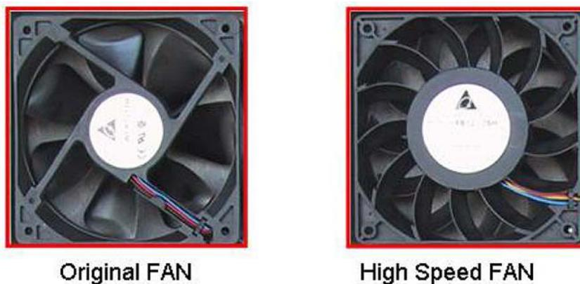
For operational purposes, the fans in the right column in Table 3 must be used with the Supervisor Engine 32.
