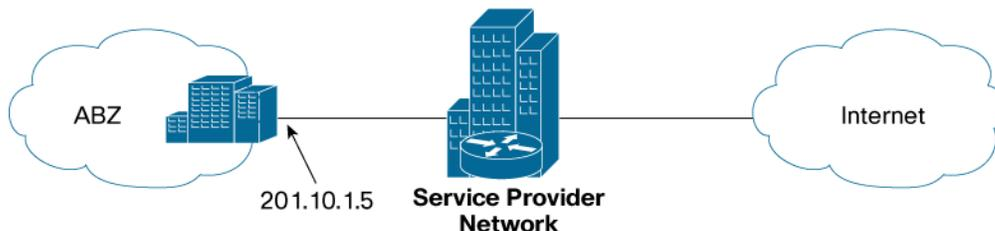
UBRL is configured in a similar way to a microflow policer. The configuration starts with the definition of a set of classification criteria using an ACL. The customer's IP address is 201.10.1.5, so the ACL is initially defined as follows:
